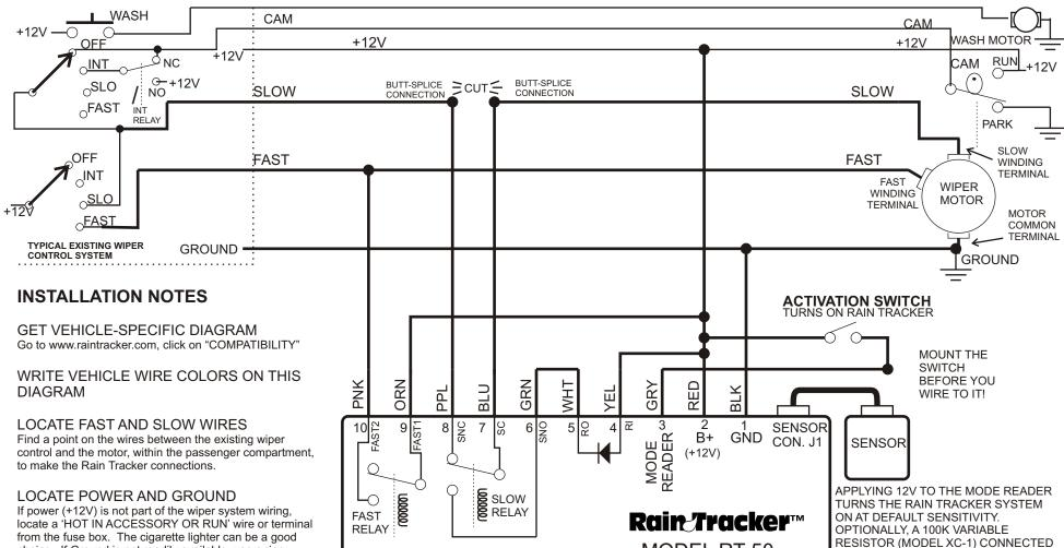
from the fuse box. The cigarette lighter can be a good choice. If Ground is not readily available, use a ring connector to connect to a good chassis ground. Scrape away paint if needed to insure a good ground.
