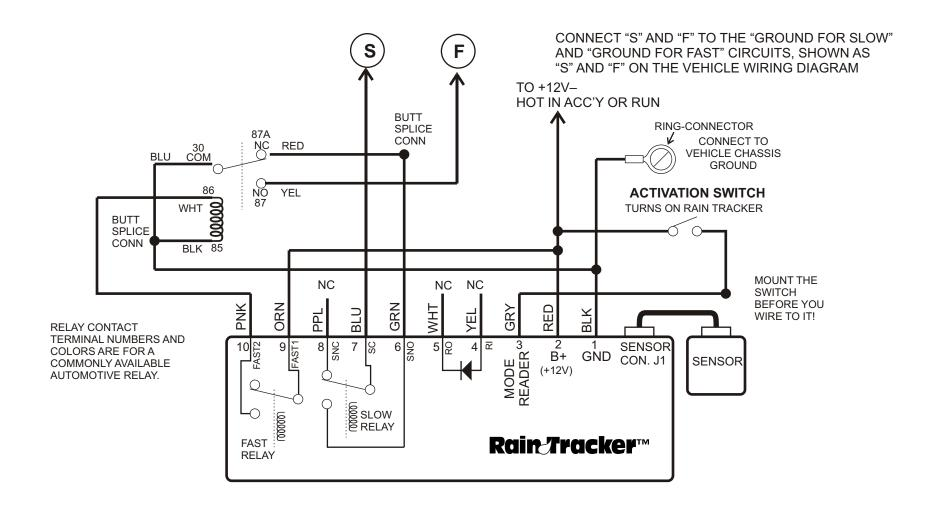
Rain Tracker Wiring Diagram:
