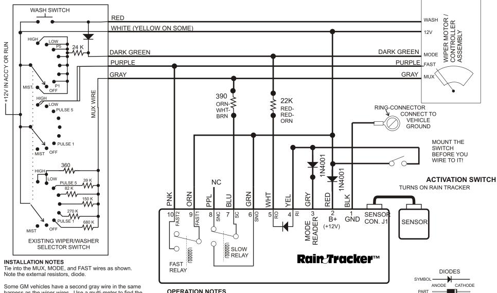
harness as the wiper wires. Use a multi-meter to find the one that cycles over several volts when the switch is intermittent mode. That wire is the MUX wire. All of the wiper wires are fairly heavy gage-- not the thinner wires of the cruise-control.
