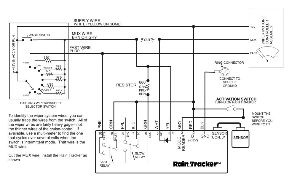
RAIN TRACKER INTERFACE WIRING DIAGRAM WIPER SYSTEM CLASSES:
