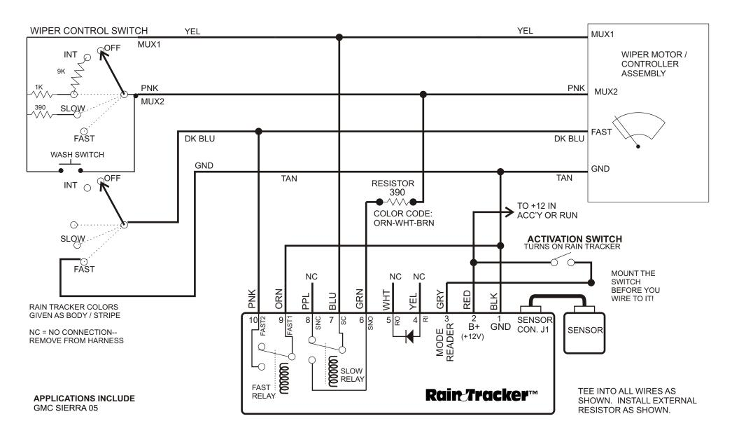
RAIN TRACKER INTERFACE WIRING DIAGRAM WIPER SYSTEM CLASS:
