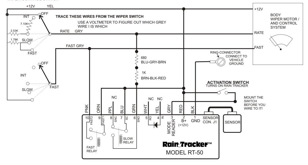
RAIN TRACKER INTERFACE WIRING DIAGRAM
