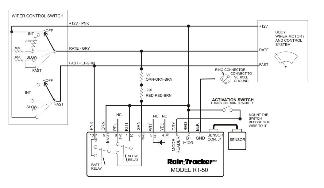
RAIN TRACKER INTERFACE WIRING DIAGRAM
