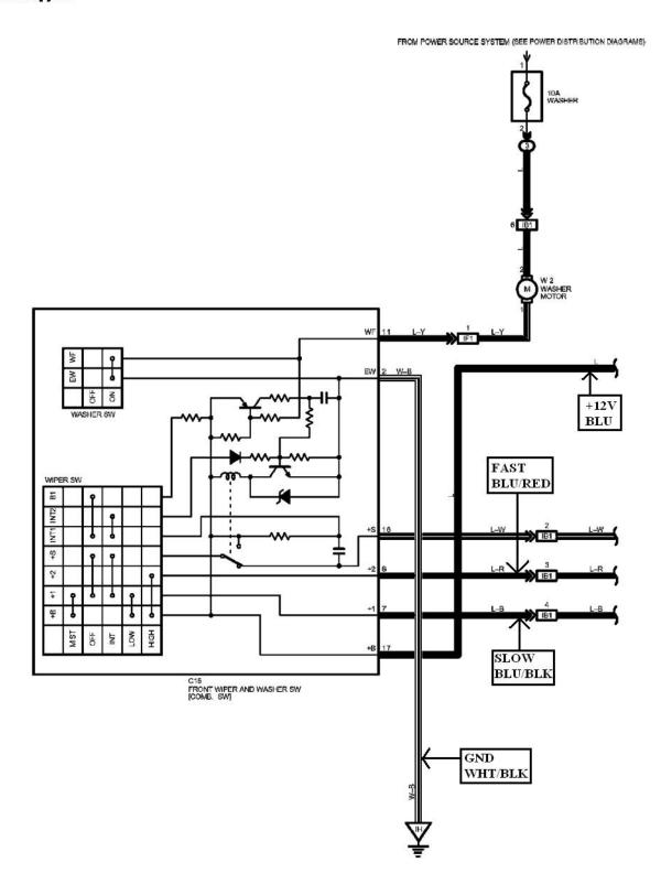
WPERS RUN WHEN 12V APPLIED TO WPER MOTOR SLOW OR FAST TERMINALS. MOTOR COMMON AT GROUND.
