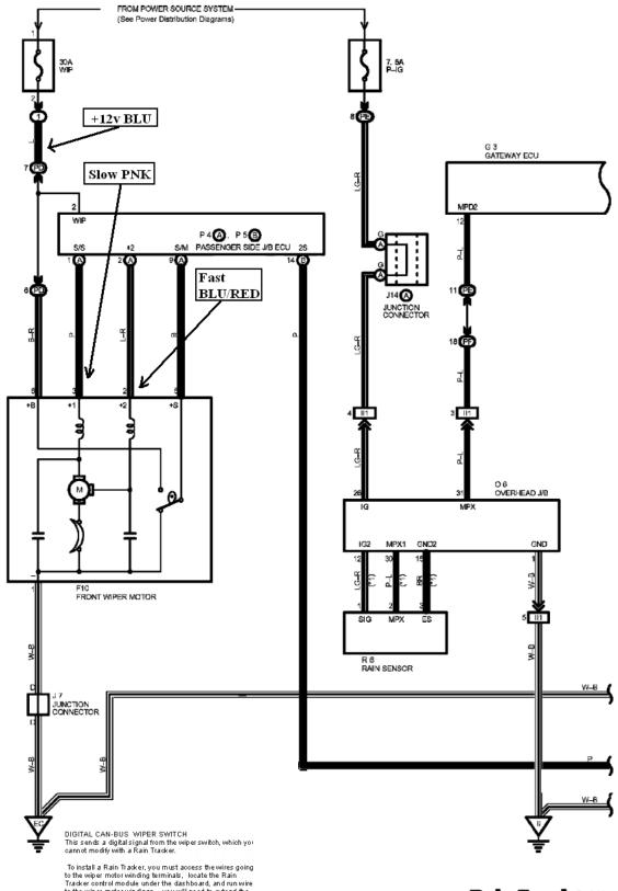
To install a Rain Tracker, you must access the wires going to the wiper motor winding terminals, locate the Rain Tracker control module under the dashboard, and run wire to the wiper motor windings—you will need to extend the wires from the RainTracker, and go through the firewall.
