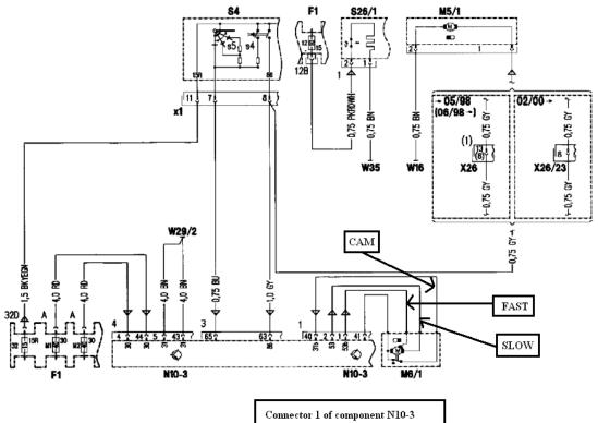
Connector 1 of component N10-3 (Combination Control Module) shows PIN 1 as FAST, PIN 2 as SLOW and PIN 40 as CAM.
