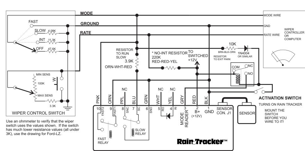
This drawing is for vehicles that have depressed park. That is, when the wipers are off, they move to a lower position below the hood.
