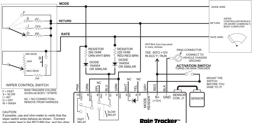
wiper switch wires behave as shown. Connect one meter lead to the RETURN line, and the other in turn to the RATE and MODE lines. With the vehicle off, you should read resistances that are somewhere near the values shown in the drawing above.
