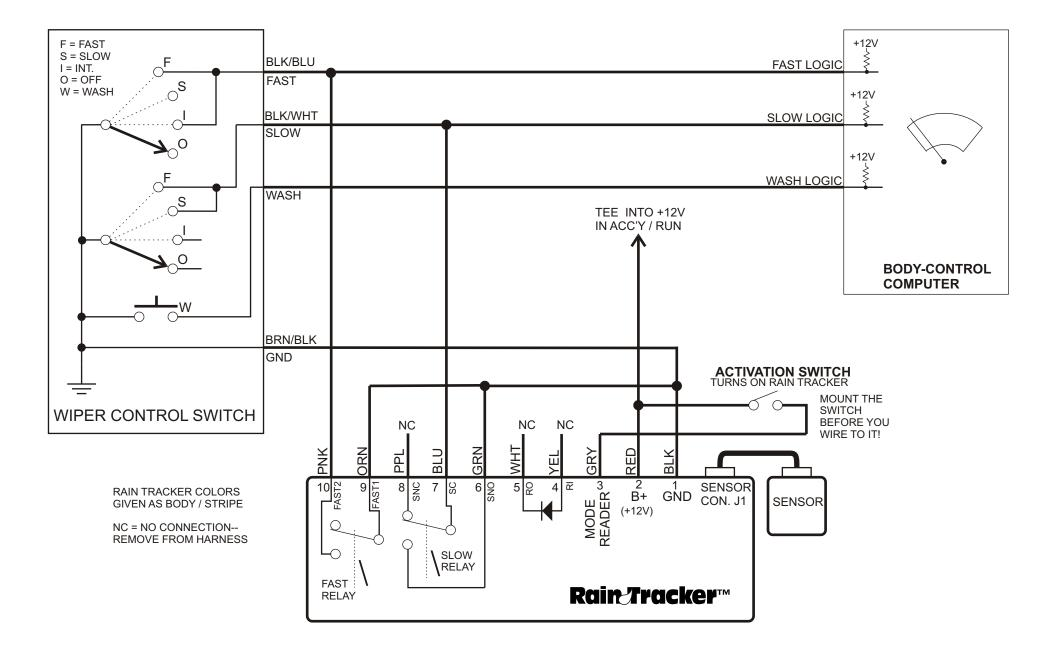
RAIN TRACKER INTERFACE WIRING DIAGRAM WIPER SYSTEM CLASS:
